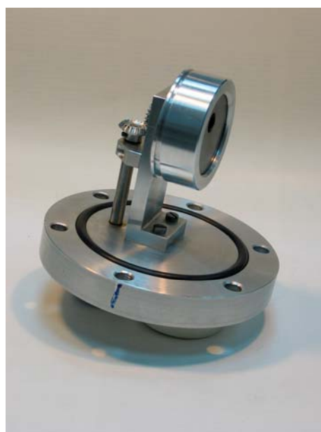
Fig. 1. Special irradiation chamber, enabling to irradiate different places on the surface of a studied crystal without necessity of opening.
