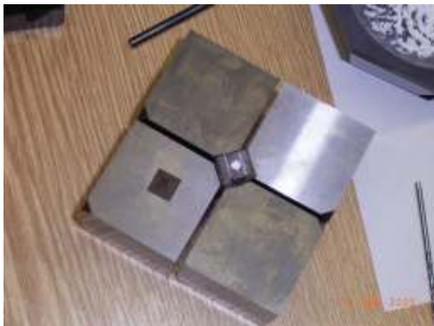
Figure 3. Four tungsten carbide anvils: the lower part mounted with a sample in external octahedral anvils.
