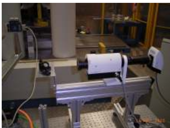
Figure 6. X-Radiography: the Ce:YAG-crystal converts an X-ray shadowgraph to an optical image. The image is magnified by the microscope, captured by a CCD-camera and finally saved on PC's hard drive. For transmission, Fire-Wire controllers and four repeaters are used. Because of the long cables the images are saved at a PC's hard drive outside the hutch.
