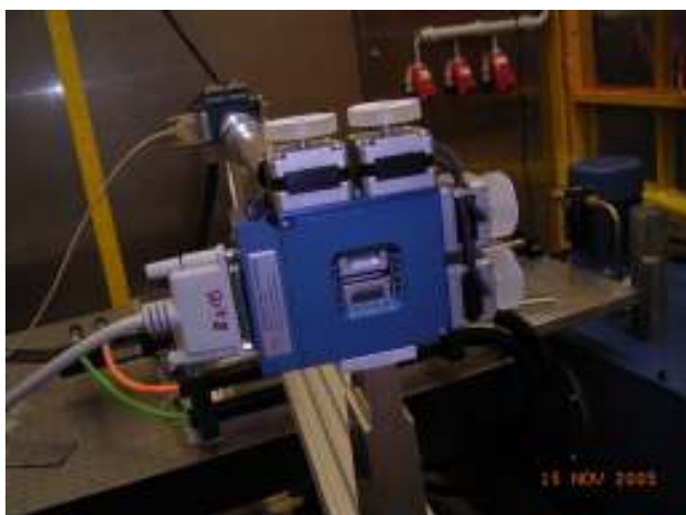
Figure 3. Slit-system with motor driven high precision slits in a distance of 1000 mm from each other to block scattered radiation and diffracted X-rays from non-sampled parts of the set-up. The distance between first slit-system and centre of the sample is 1200 mm.
