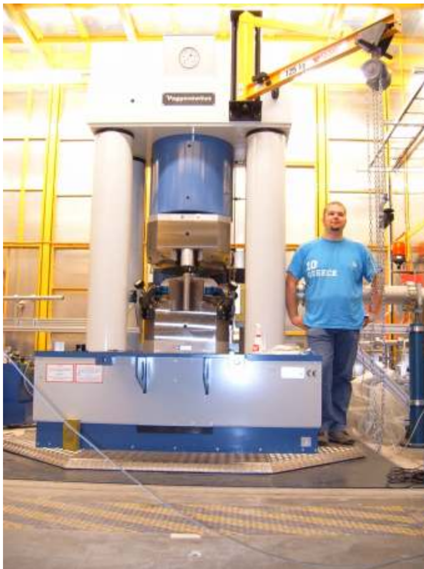
Figure 1. MAX200x surrounded by aluminium-lead aluminium hutch at the HARWI-II hall. The synchrotron beam position in the HARWI-II – Hall is only 1200 mm above the ground. Thus the multi-anvil press had to be put into a cavity of 3700 mm length, 3220 mm width and 140 mm depth. A 500 mm thick foundation of concrete had to be poured in order to support the weight of 30 tons. This press has a maximal load of 1750 tonnes. It is rotatable \pm 15^\circ , moveable \pm 125 mm in z -direction and \pm 50 mm in x -direction.
