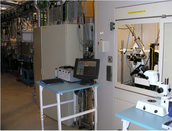
Figure 3. The experiment hutch of the MAD station at I911. The kappa goniostat can be seen through the open hutch window. The setup with sample microscope (to the right), the fast and easy access to the goniostat through the hutch window, the sample alignment interface (the touch screen on the left) and the close access to the control room (2-3 m) forms a very convenient environment for the user.
