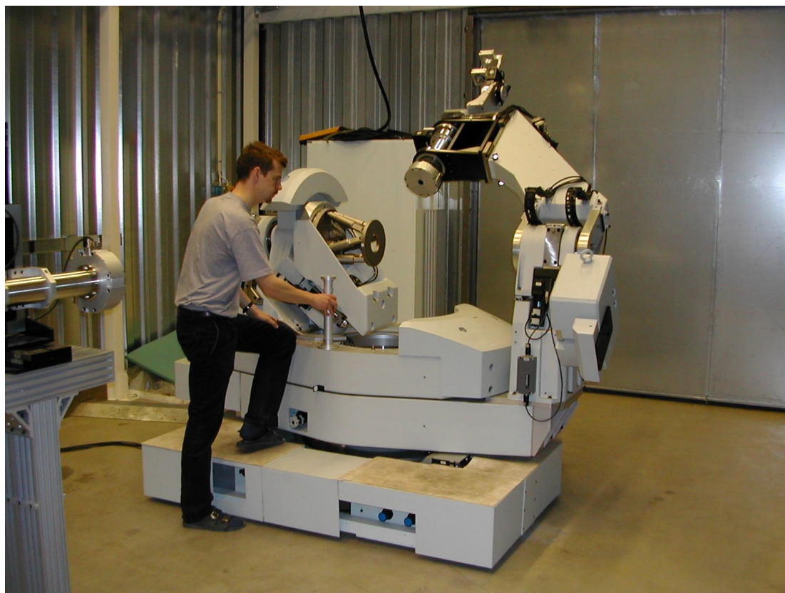
Figure 2. The Newport/Micro-Controle x-ray diffractometer at I811 shown in the “kappa” configuration. The sample/UHV-chamber is aligned using a Physik Instrumente hexapod system and the detector arm is equipped with slit system, goniometer for analyzer crystal and a scintillation detector.
