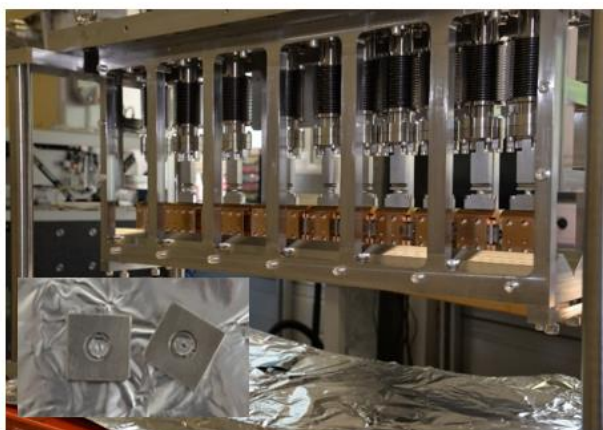
Figure 1. Horizontal transfocator and beam through a 20 \mu\text{m} pinhole.
