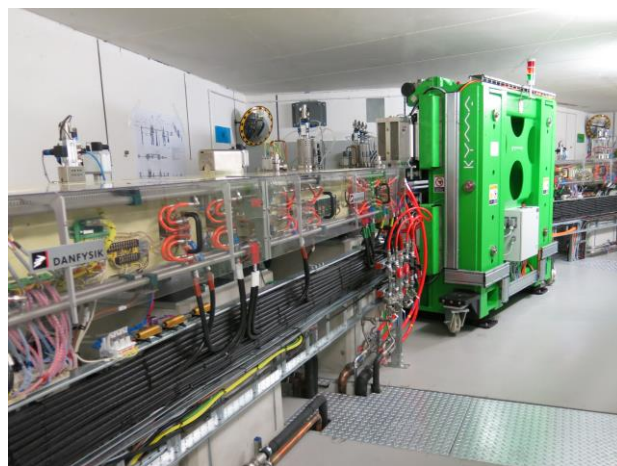
Figure 1. Inside SOLARIS storage ring tunnel: double bend integrated achromats and UARPES beamline undulator.
