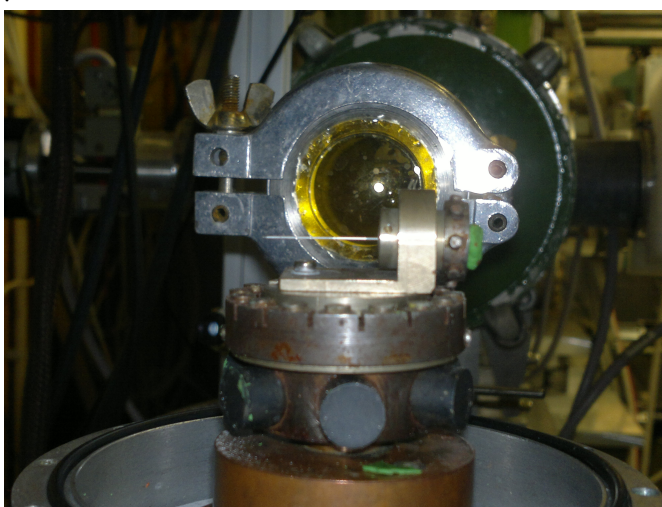
Figure 1. The capillary inside the cryostat prepared for low-temperature X-ray diffraction measurements (the upper part of the cryostat was removed).
