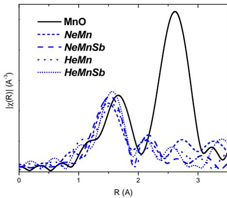
Figure 2. Magnitude of Fourier transform of the EXAFS spectra of the samples annealed at 350°C compared with the MnO standard.
