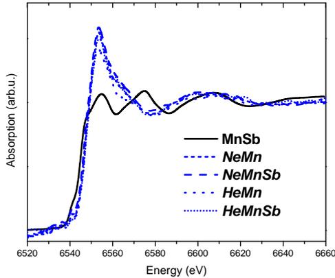
Figure 1. XANES of the samples annealed at 350°C compared with MnSb standard spectrum.
