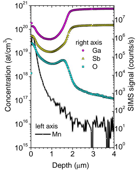
Figure 3. SIMS depth profiles of the element distribution in the *NeMnSb* sample annealed at 350°C.
