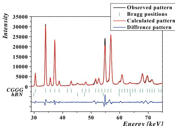
Figure 1. Le Bail refinement plot of the calcium gallium germanium garnet, sample after compression without pressure. The vertical bars refer to peak positions for CGGG and hBN.
