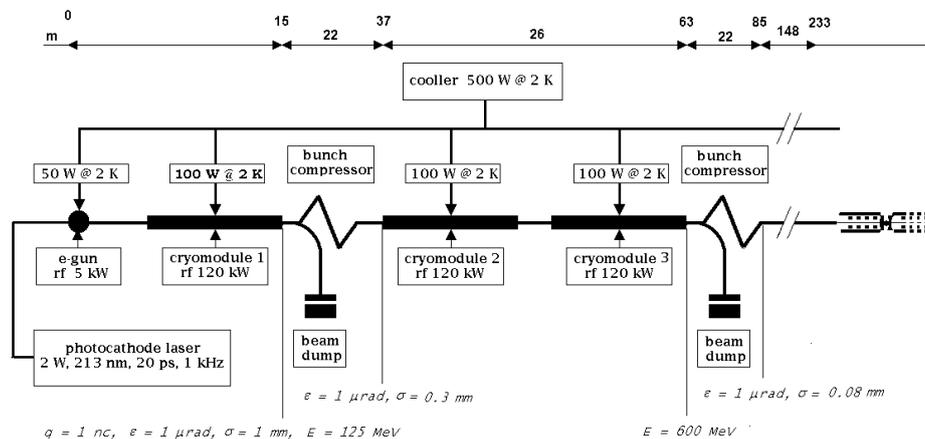
Figure 2. Conceptual drawing of POLFEL linac.
