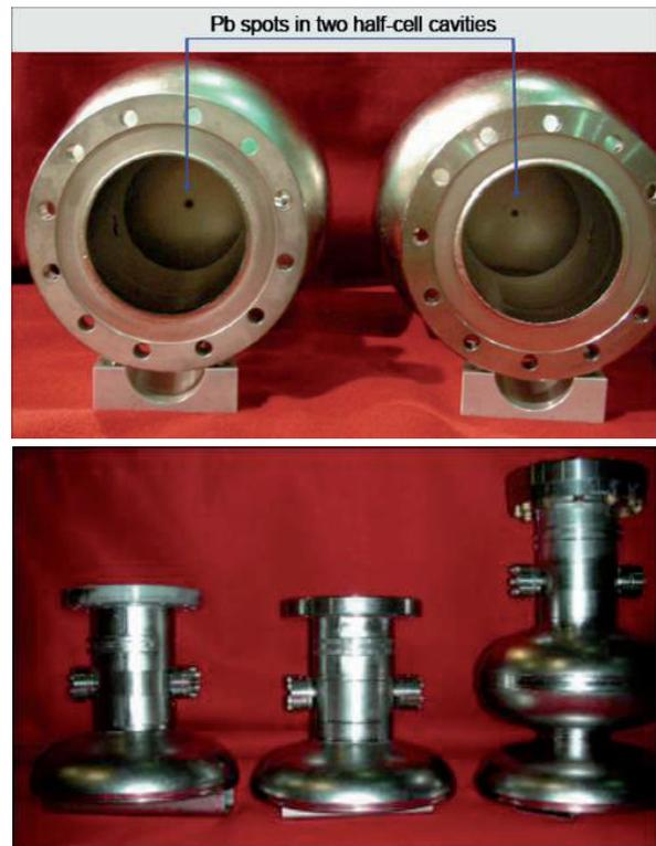
Figure 1. Superconducting electron guns. Upper picture shows lead photocathode spots deposited onto back wall of resonant cavities. The lower picture shows 0.5 and 1.6 – cell acceleration structures.
