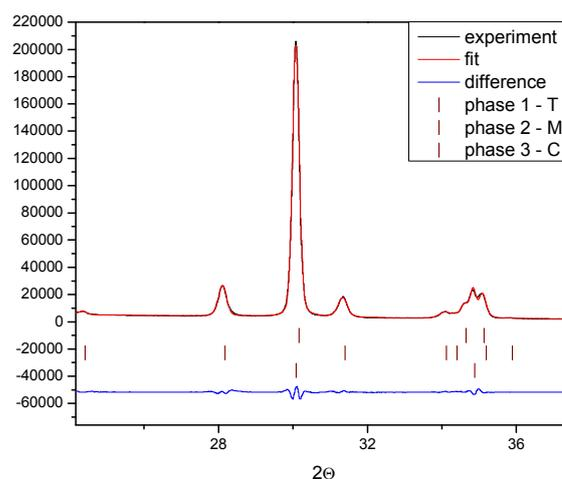
Figure 1. Experimental X-ray diffraction patterns of Pr-doped YSZ (4.79 mol % of yttria). The vertical bars show the peak positions for the tetragonal phase (upper), monoclinic phase (center) and cubic phase (lower).
