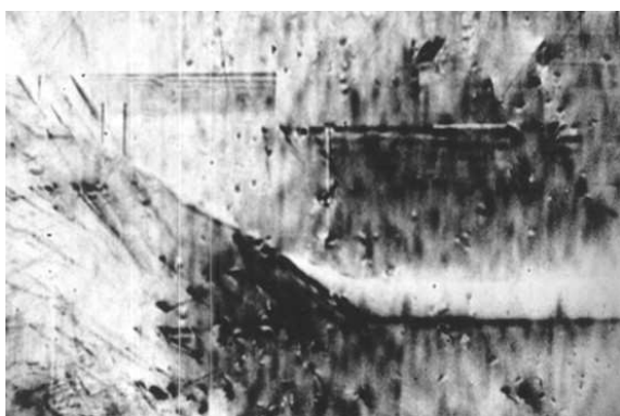
Figure 5. The back reflection (Bragg-case) synchrotron double-crystal topograph of (001) oriented diamond plate in 113 reflection of 0.154 nm radiation revealing interference fringes in images of the two stacking faults [7].
