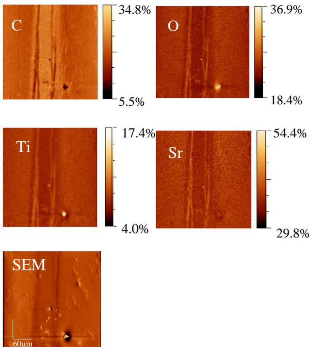
Figure 1. The AES chemical distribution maps for carbon, oxygen, titanium and strontium of the contact area with the electrode for the Fe doped STO film. The SEM image of the analysed area was added.
