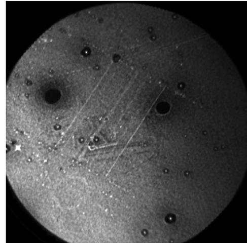
Figure 2. The LEEM image of 2% Fe doped STO film recorded from the area with the diameter of 20 micrometers. The white parallel lines are the effect of earlier contact with the biased AFM tip.
