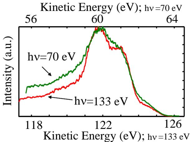
Figure 3. The photoemission spectra obtained with two various photon energy from electro-modified by AFM tip area.
