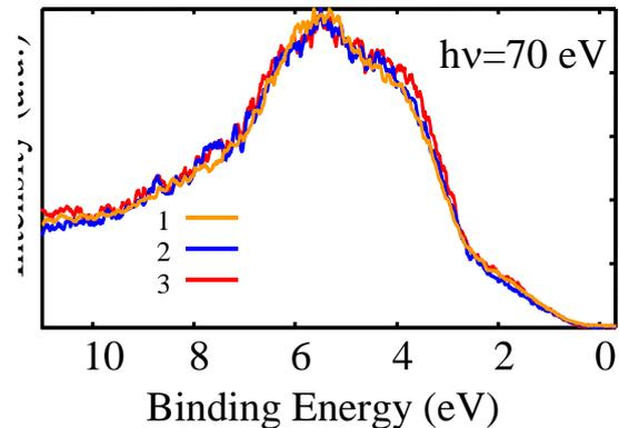
Figure 4. The valence band spectra recorded for: 1 – area electroformed by the biased AFM tip, 2 – outside electroformed area, 3 – after annealing at 120 °C.
