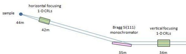
Figure 1. Optical layout of ID15B.
