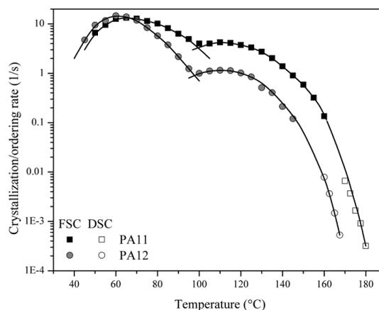
Figure 1. FSC-based crystallization rate of PA11 and PA12.
