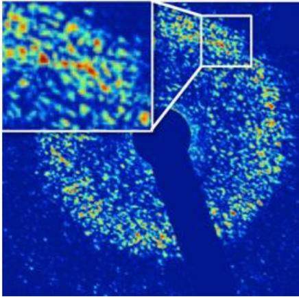
Figure 1. Typical pattern showing randomly oriented speckles.
