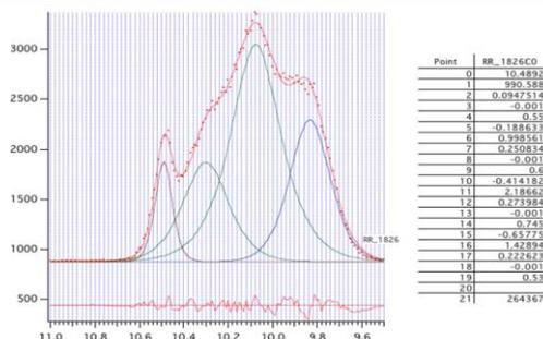
Figure 2: Spectrum taken with 4.6 eV  $E_{\text{phot}}$  for 6 Å Ag film.
