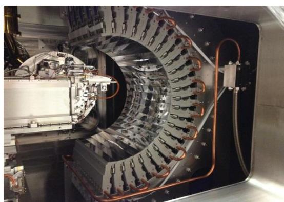
Figure 1: Pilatus 12M detector in I23 vacuum vessel.
