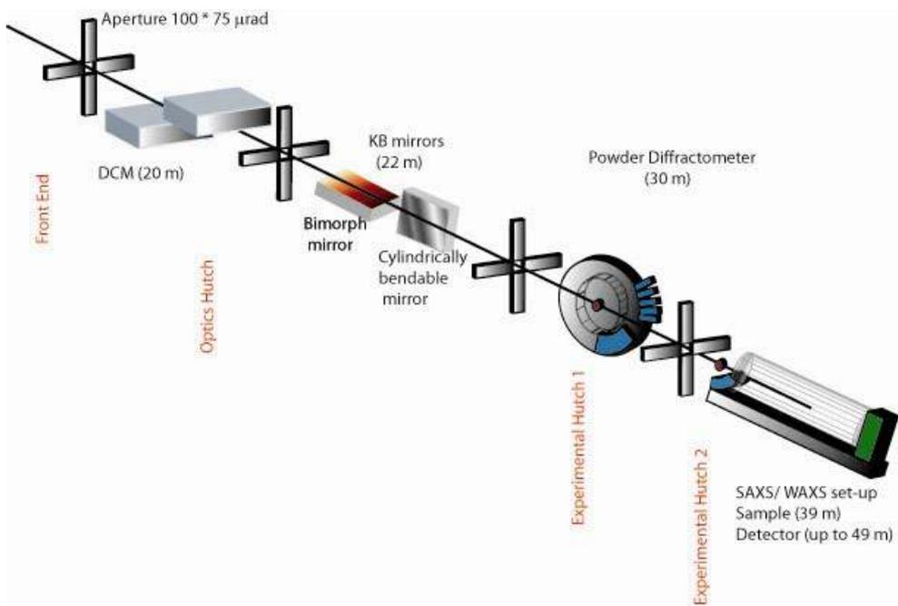
Figure 3. The general layout of the proposed combined powder diffraction and SAXS beamline.
