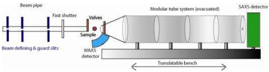
Figure 5. The SAXS/ WAXS set-up in experimental hutch 2.
