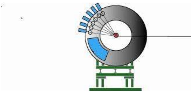
Figure 4. The high-resolution powder diffractometer with several analyser crystals/ scintillation counters and a rapid PSD detector at negative  $2\theta$  for kinetic studies.
