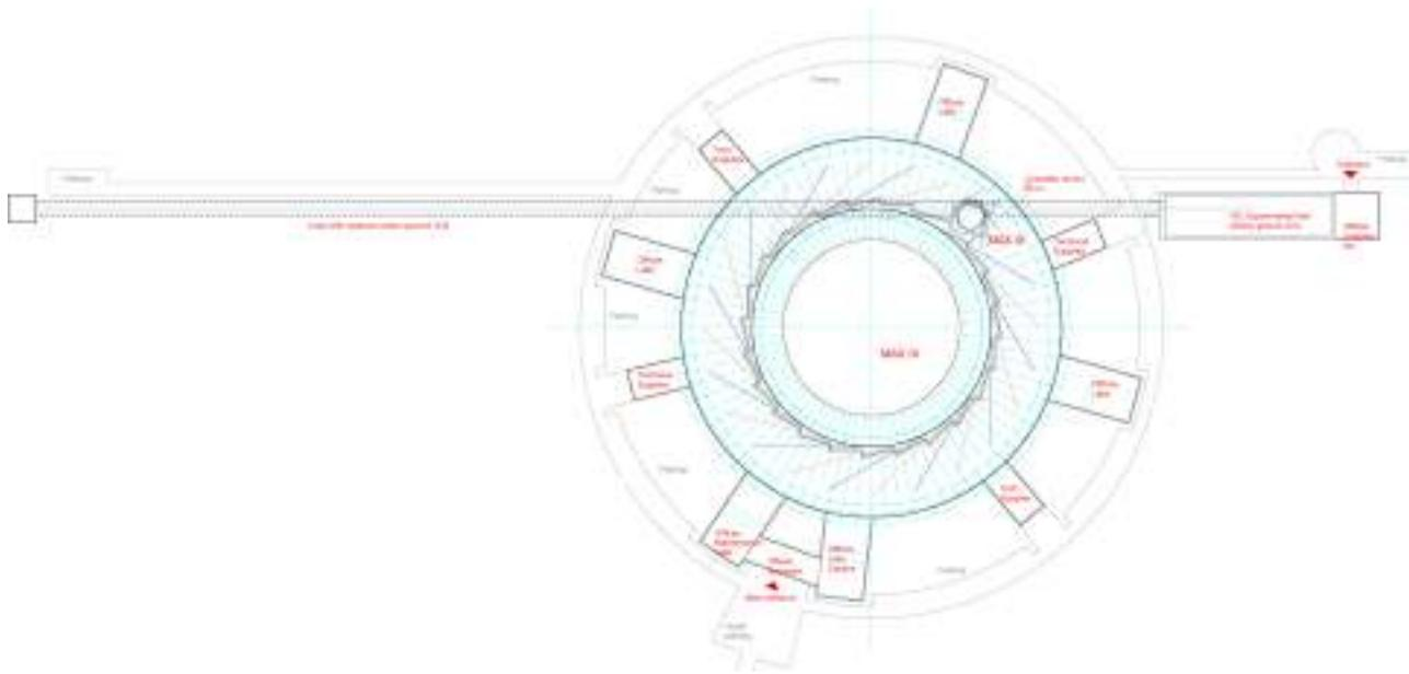
Figure 1. The proposed MAX IV facility with a several hundred meters long linac for injecting the three storage rings and for feeding a FEL (Illustration from the Conceptual Design Report of MAX IV).
