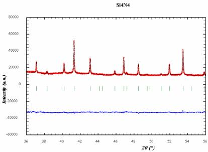
Figure 1. Rietveld refinement result in a broad angular range for the c-Si3N4 ceramics (upper panel). Experimental - crosses, calculated - solid line. The difference pattern is shown below the powder pattern. The lower panel (a magnified part of the upper one) illustrates the high quality of the fit.
