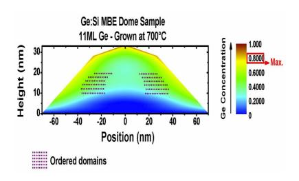
1) In the system Ge on Si, we show how the 3D chemical composition can be determined within dome-shaped GeSi islands. In addition, from the measurement of "forbidden reflections" the atomic ordering of the GeSi alloy, forming the dots, can be quantified. These results are obtained using the model of Iso-Strain-Scattering for data evaluation.
