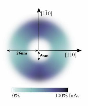
2) This approach breaks down for InAs islands which form quantum rings after MBE overgrowth with GaAs. From Finite Element Modelling of the experimental intensity maps in reciprocal space close to the (2-20) and (220) surface reflection, we reveal a highly anisotropic In distribution within the rings (see figure). From grazing incidence small angle scattering (GISAXS) the ring morphology is found to be of circular symmetry.
