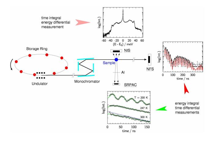
Figure 1. Schematic layout of a NRS experiment.
