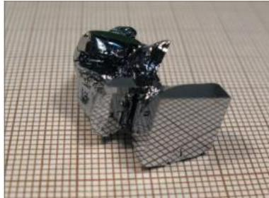
Figure 1. A monocrystal of Pb<sub>0.77</sub>Sn<sub>0.23</sub>Se obtained by the self-selecting vapour growth method.
