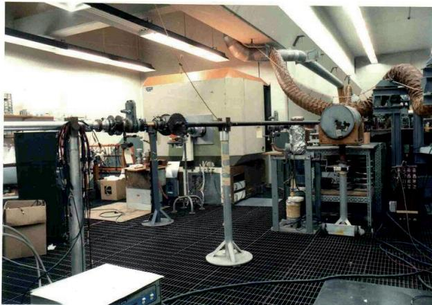
Figure 1. At the back there is VdG accelerator. On the left – PIXE line, on the right – microbeam line.
