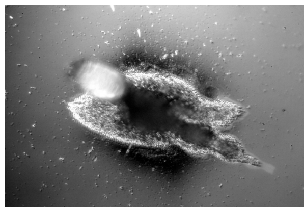
Figure 2. Ablation crater created on Si surface by a few shots of femtosecond free-electron laser pulses (interference-polarizing microscope with Nomarski contrast).
